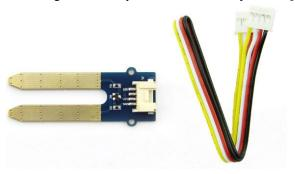
Figure 12: Soil Moisture Sensor [12]
